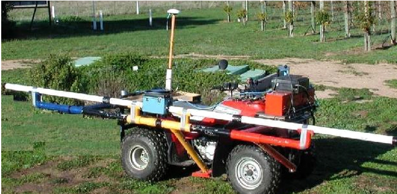
Rapid electromagnetic profiling system similar to that used by Douglas Partners at Menangle Park which comprised quad bike, Geonics EM31 Ground Conductivity Meter, Fugro Omnistar DGPS and Psion data logger.
